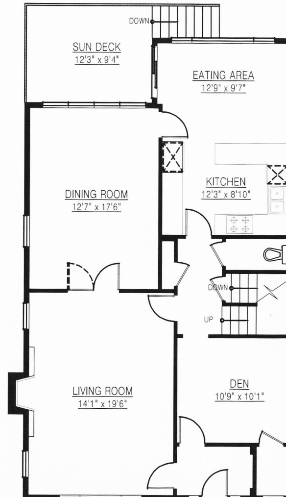
MAIN FLOOR PLAN FLOOR AREA: 1097 sq.ft. SUN DECK AREA: 118 sq.ft.
